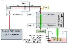
Fig. 1 Schematic representation of the integrated OCT system and the cultured muociliary epithelium sample. SMS: Scanning mirror system; DM: Dichroic mirror
