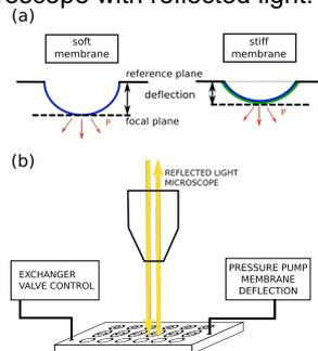
Fig. 1 Schematic representation of the measurement setup.
