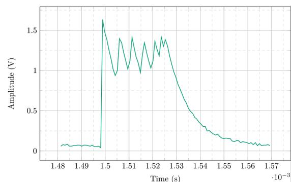
Figure 2 Received data pulses, measured at the output of the envelope detector
