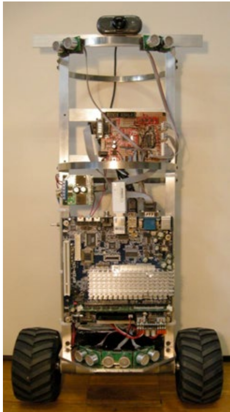
Fig.1, A first prototype of a self balancing autonomous robot with a low power PC, a microcontroller for real time processing and many sensors.
