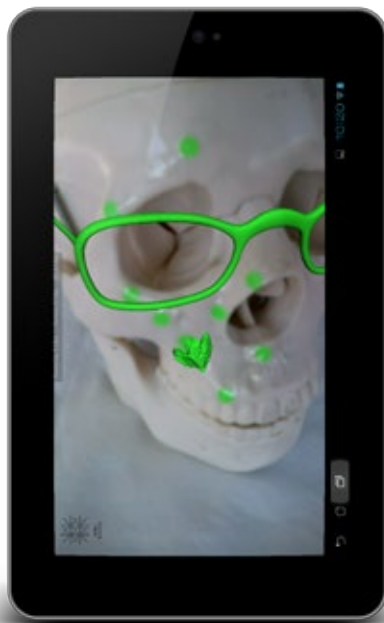
Figure 1 Augmented reality - the skull is a real world object; the tumor and the glasses are virtual objects; occlusion object (skull) is enabled thus portions of the tumor within the bone are not visible
