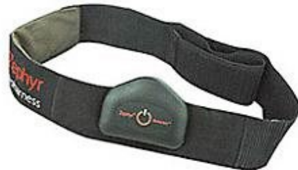
Fig.2, The bioharness from Zephyr is a chest belt which measures the heart rate, breathing rate, movements and body temperature. It sends this information to the robot over Bluetooth. Source: Zephyr-technology.
