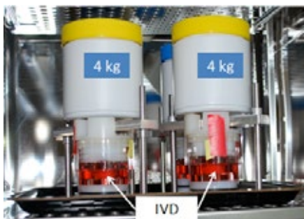
Fig. 1 Loaded IVDs in custom-made chambers in 37°C incubator at 5% CO 2 . Disc were previously injected with MMP-3, ADAMTS-4 and HTRA1 and PBS as a control and cultured for 8 days with a period of diurnal loading (0.4MPa for 16h, no load for 8h).
