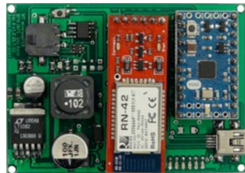
Figure 1 30 V Stimulator providing two channels. Bluetooth module (red) microcontroller (blue).
