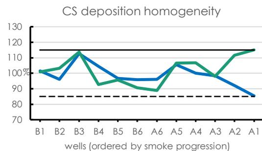
Fig. 2 Relative cigarette smoke deposition between wells (n=2). Acceptance range ( $\pm 15\%$ ) indicated by the CF-AX12 manufacturer.
