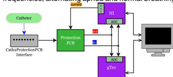
Fig. 1 Simultaneous sampling of ECG and impedance through a multipurpose and a reference device
