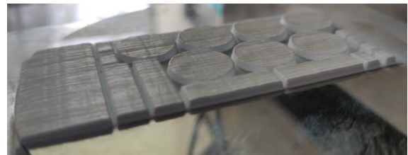
Fig. 2 Printing batch produced on a wax base layer used for mechanical characterization
