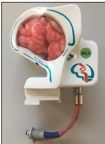
Fig. 1 Example of an assembled patient-specific aneurysm training phantom model.
