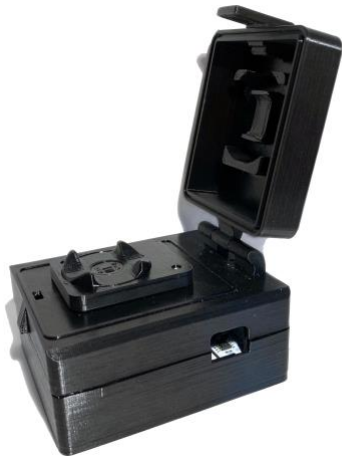
Fig. 1 Final PPG simulator design used for testing with Aktiia's sensor.
