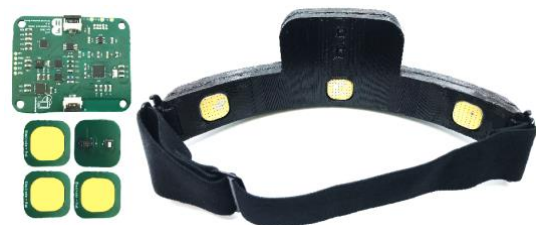
Fig. 2 The prototype consists of the overall electronics, sensors, flexible housing, an elastic band.
