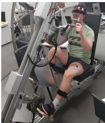
Fig. 1 Participant cycling with EEG measurement on the Bi-Pedal device from the rehaLab, BFH
