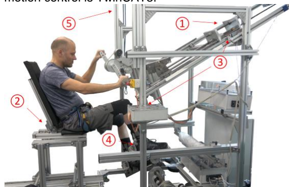
Fig. 1. The Functional Movement Stimulator (FMS). ① Arm drive sliding system, ② seat system, ③ safety components, ④ orthoses, and ⑤ body support frame.
