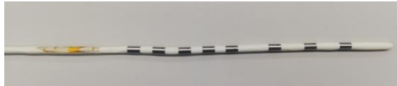
Figure 1: Catheter prototype with eight ECG electrodes and a NIRS sensor with two LEDs and a phototransistor.
