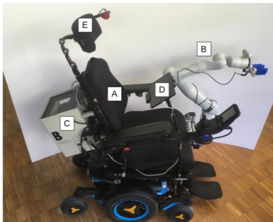
Fig. 1: Test system. (A) electric wheelchair, (B) robot arm, (C) control electronics, (D) tablet, (E) head pressable stop switch. Components (D&E) are most relevant for this thesis.
