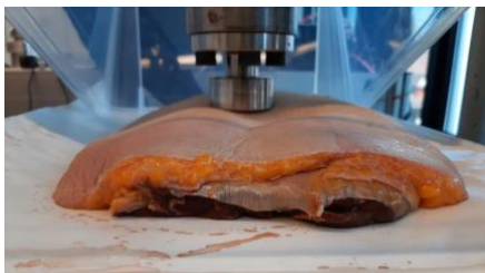
Fig. 1 A trochanteric soft tissue sample tested with a flat, cylindrical indenter on the MTS testing system.
