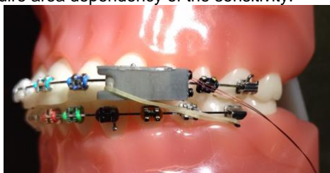
Fig. 1 The final sealed prototype with an FSR sensor inside, attached to fixed braces.
