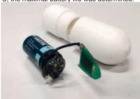
Fig. 1 The developed wireless sensor attached to its ½ AA lithium battery next to the 3D-printed capsule implant.
