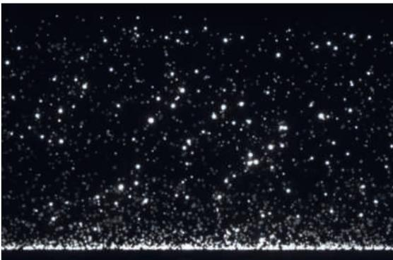
Fig. 1: One particle image of the flow inside the in vitro ureter model
