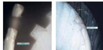
Fig. 3 Microscope pictures of the microholes after thermobonding. On the left, a delaminated FPCB and on the right, a laminated FPCB.
