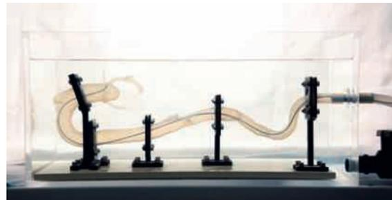
Fig. 2 Final setup of the training and testing simulator for PTCA balloon catheters. The silicone models consist of Elastosil Vario 15A.
