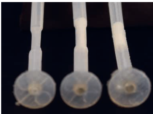
Fig. 1 Different stenosed arterial phantoms based on a generalized geometry
