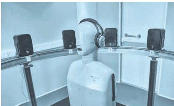
Head and torso simulator for electroacoustics tests of audio devices, microphones, headphones, hearing aids, hearing protectors and smart speakers.
