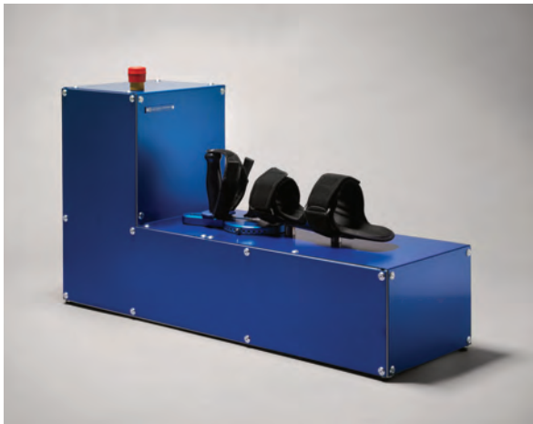
Case-study of a technical device to measure wrist rigor (University of Berne & Lutz Medical Engineering GmbH).
