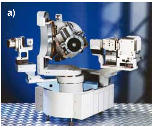
HRXRD equipment used for RSM investigations (a), encapsulated resonator MEMS (b), schematic view of the HRXRD experiment (c).
