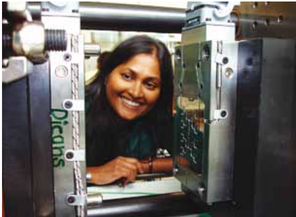
Inspection of the new mold installed in the injection molding machine (Arburg 320 Allrounder).
