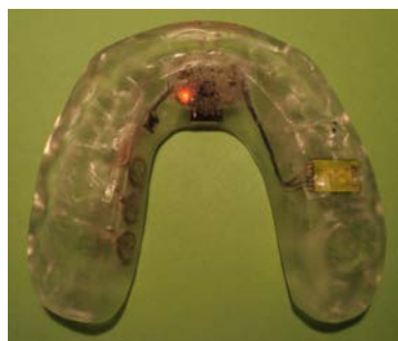
Active mouthguard with sensor and transmitter electronic and batteries
