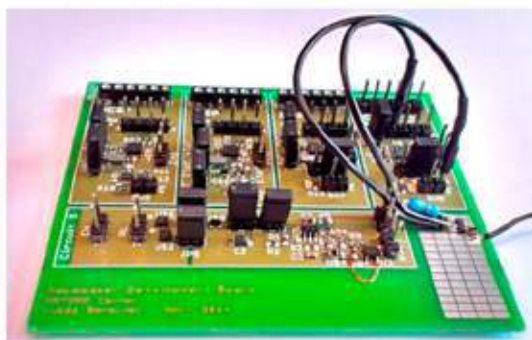
Fig. 1 Development board with microcontroller based circuits for an endocardial pacemaker and an analog circuit for a lead- and batteryless epicardial pacemaker
