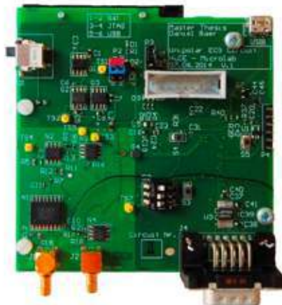
Fig. 1: Evaluation board containing the unipolar analog front-end and a microcontroller to measure a surface biopotential.
