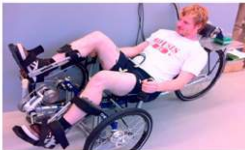
Fig. 1 FES tricycle test bed in use
