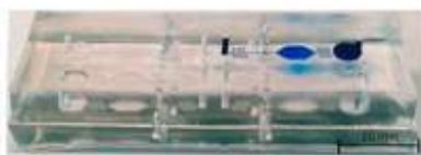
Fig. 2: Fabricated PDMS microfluidic chip including the new pumping system. One fluid channel is colored with blue food dye.
