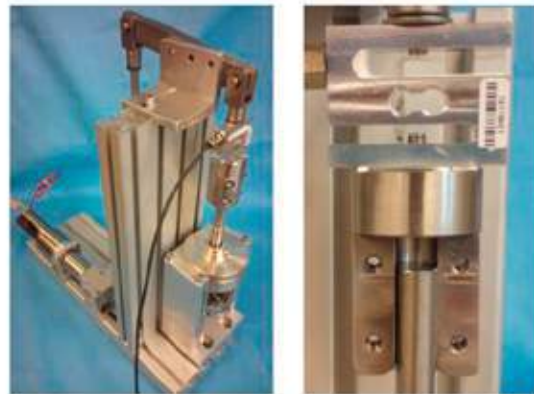
Fig. 2 a) Assembled device with motor block in back, sample chamber in front, force measurement adjacent to sample to minimize errors. b) Force measurement load-cell with open insertion mechanism, flexible height depending on sample geometry.
