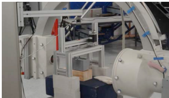
Fig. 1 Experimental set-up for fluoroscopy measurements during bone cement substitute injections
