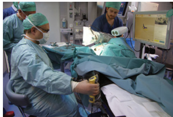
Preclinical evaluation of a new surgical robot system for minimally invasive cochlear implantation. Photo: ARTORG Center
