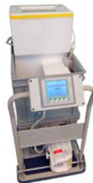
Fig. 1: The portable heart perfusion system comprising electric, perfusate, oxygen and heart modules. The system includes a touch-panel for parameter control and monitoring, and is mounted on a trolley for easy displacement.
