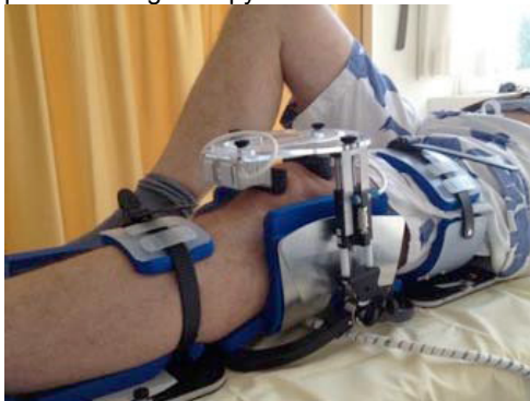
Fig. 1 Knee Rehabilitation Device (KRD) prototype developed by the ILT, University of Applied Sciences Rapperswil
