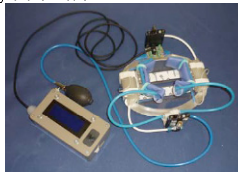
Fig. 2 Newly developed patella grippers and newly developed measurement system installed on the KRD
