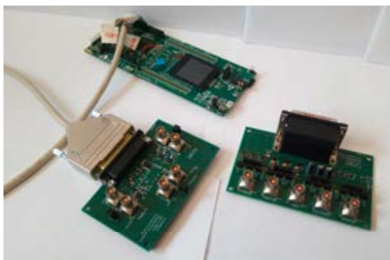
Figure 1: PCBs designed to characterize temperature sensors and accelerometers. On the right side, the accelerometer PCB. On the left side, the PCB for temperature sensor. Behind, the STM32F412ZG
