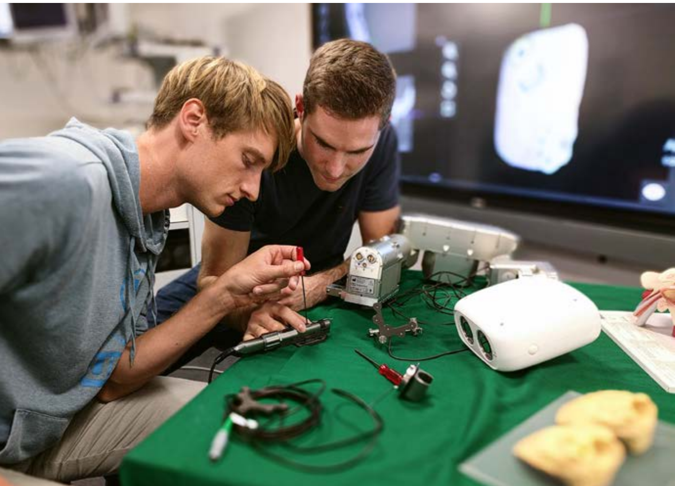
Assembly of surgical robot system for hearing aid implantation. (© ARTORG Center, University of Bern 2019)
