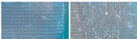
Fig. 1 Scotch test procedure to force the parylene and SiO<sub>x</sub> film delamination after ageing in an aggressive environment. Left: before scotch test. Right: after scotch test.
