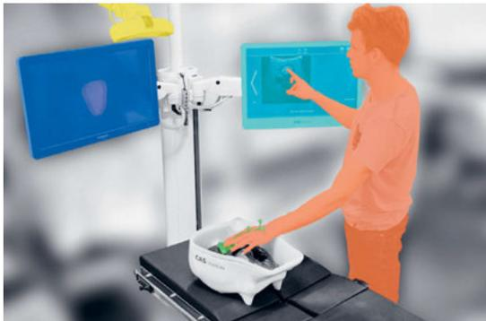
Fig. 1 The setup in the operating room: Red the surgeon; Yellow the tracking camera; Green the ultrasound probe; Dark blue the 3D screen; Light blue the 2D screen.
