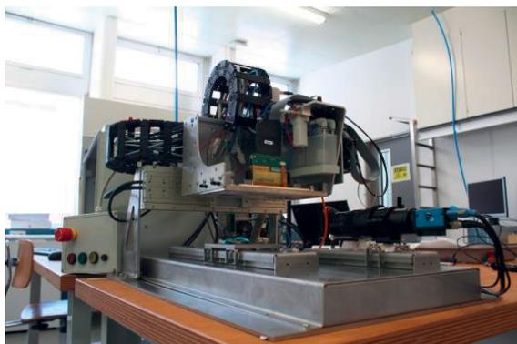
Fig. 1 Inkjet printing platform with dropwatching and a 256-nozzle industrial inkjet printhead implemented
