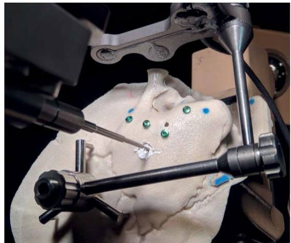
Fig. 2 The robot performs the milling task based on the planning with the developed software.
