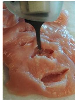
Fig. 2 Dissection test with ultrasonic microscalpel prototype on a chicken breast.
